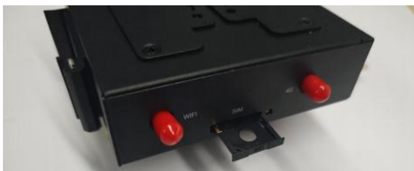
Figure 6.5.1-2 Router card slot removal diagram
