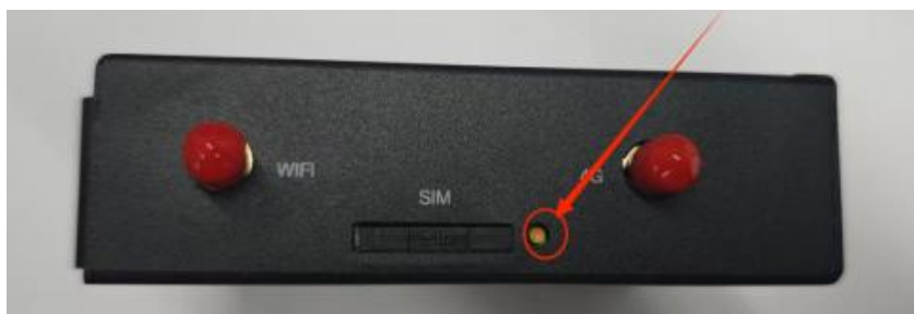
Figure 6.5.1-1 Router Card Slot Location Diagram
