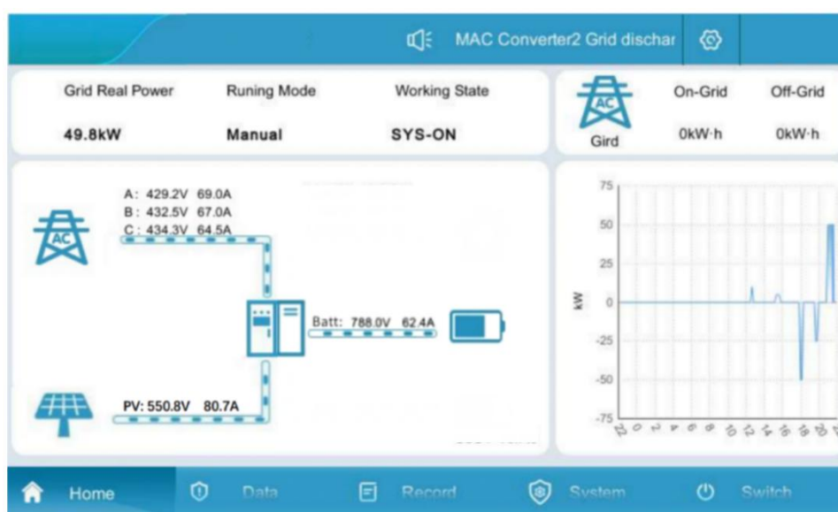
Figure 5.1 -2Main Page PV Connected.
