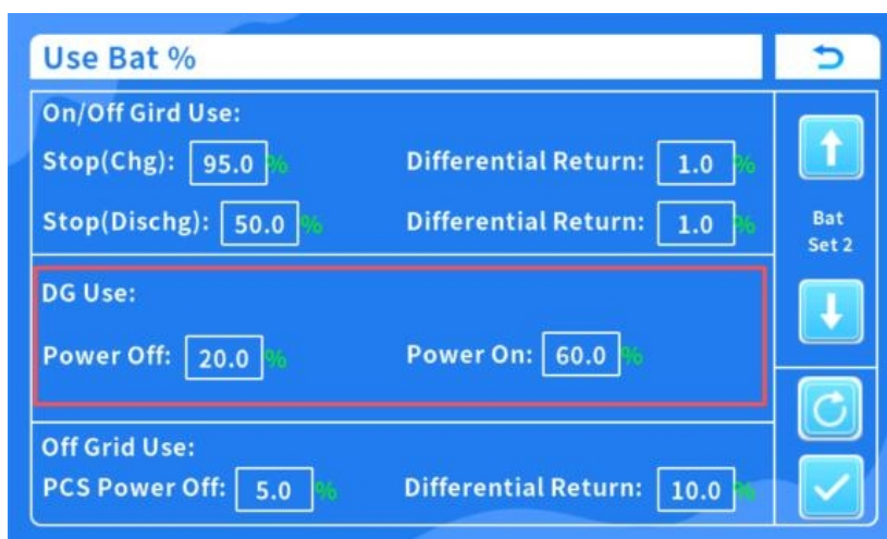
Figure 6.6-3 Generator SOC start/stop configuration
