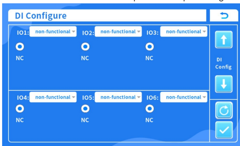
Figure 6.12.3 Input dry contact configuration page
