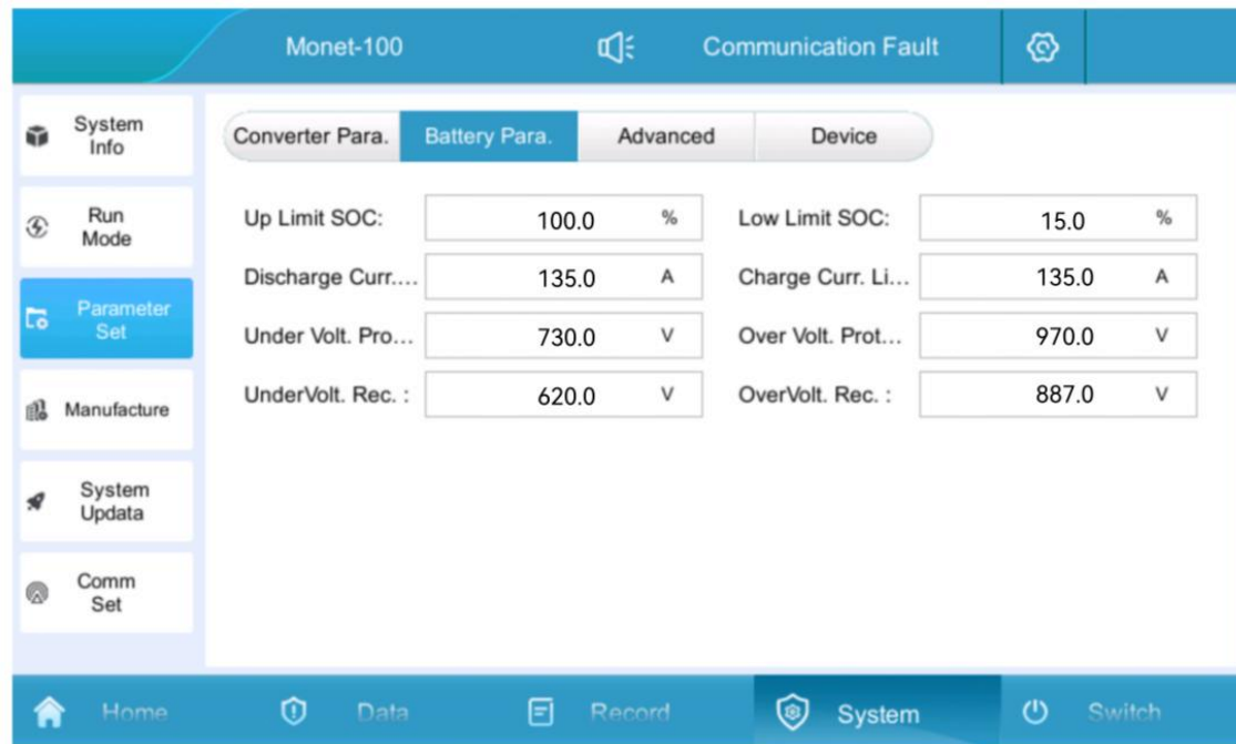
Figure5.4.5 Battery charging and discharging settings interface
