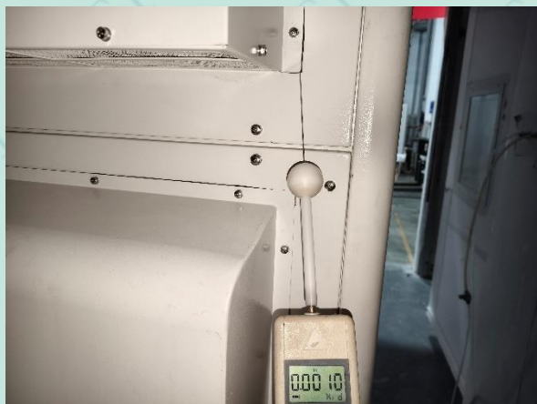
Fig 11 Fig 10 Testing of hazardous parts against contact
