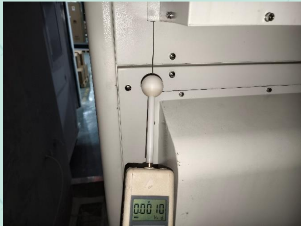
Fig 9 Testing of hazardous parts against contact
