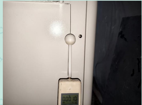
Fig 10 Testing of hazardous parts against contact
