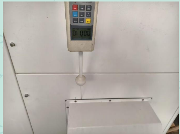
Fig 10 Testing of hazardous parts against contact
