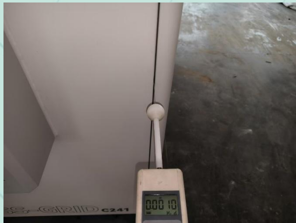
Fig 9 Testing of hazardous parts against contact
