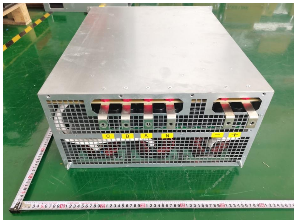
Figure 10. PCS (Power conversion system) view
