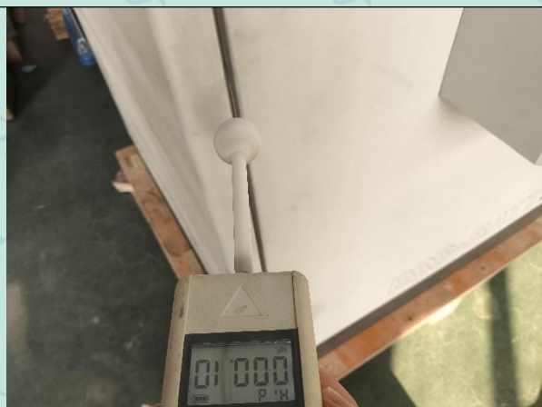
Fig 10 Testing of hazardous parts against contact
