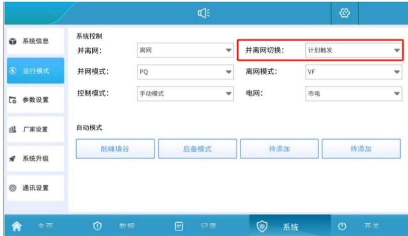
Figure 5.4.4-1 Manual on-grid and off-grid switching mode setting interface
