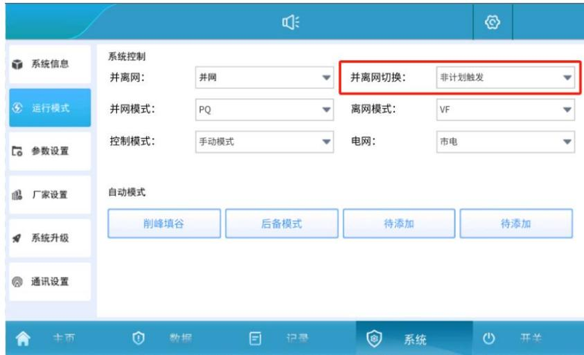
Figure 5.4.4-2 Automatic on-grid and off-grid switching mode setting interface
