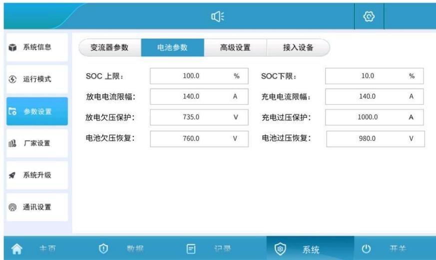
Figure 5.4.5 Battery charge and discharge settings interface
