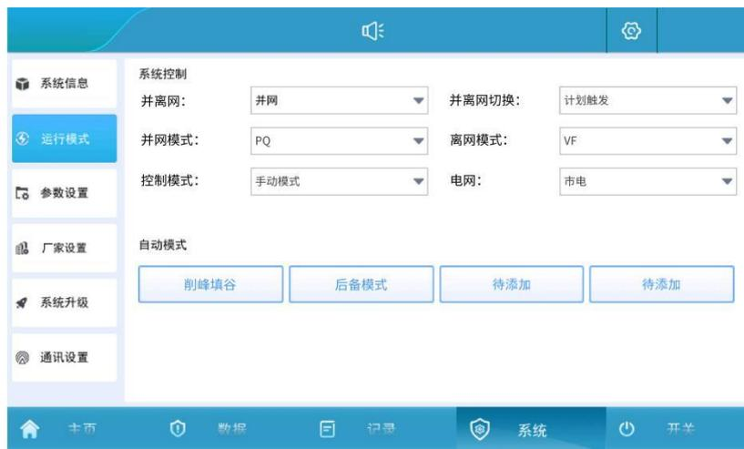
Figure 5.4.1-1 On-grid and off-grid settings interface
