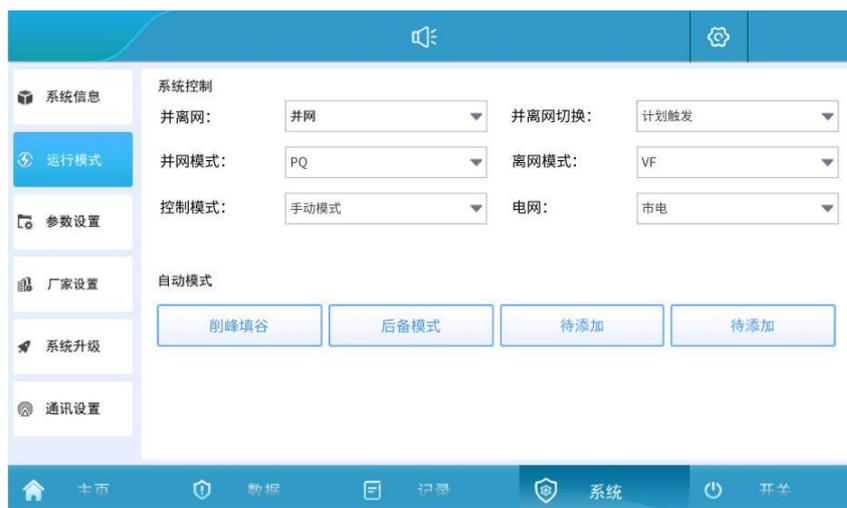
Figure 5.4.2-1 Grid-connected manual mode setting
