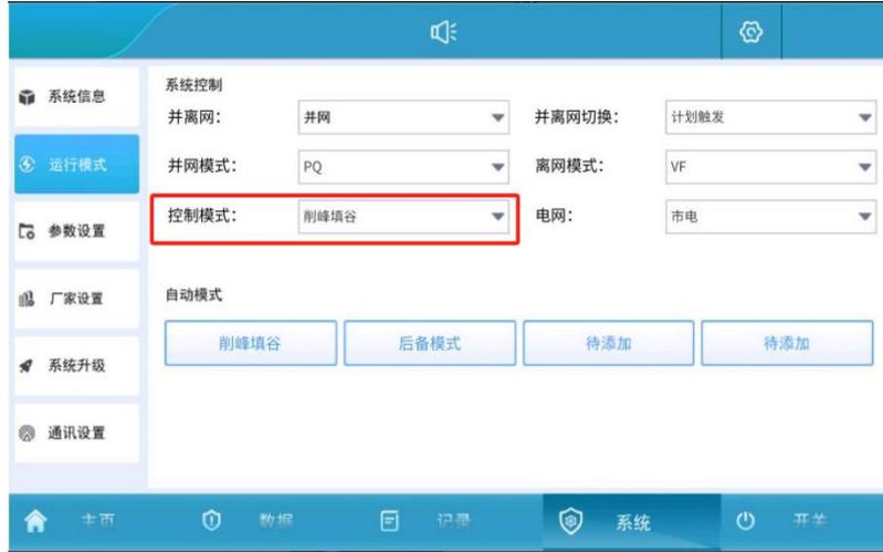
Figure 5.4.3-4 Peak shaving and valley filling control mode
