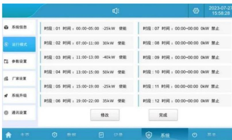
Figure 5.4.3-3 Peak shaving and valley filling charging and discharging setting
