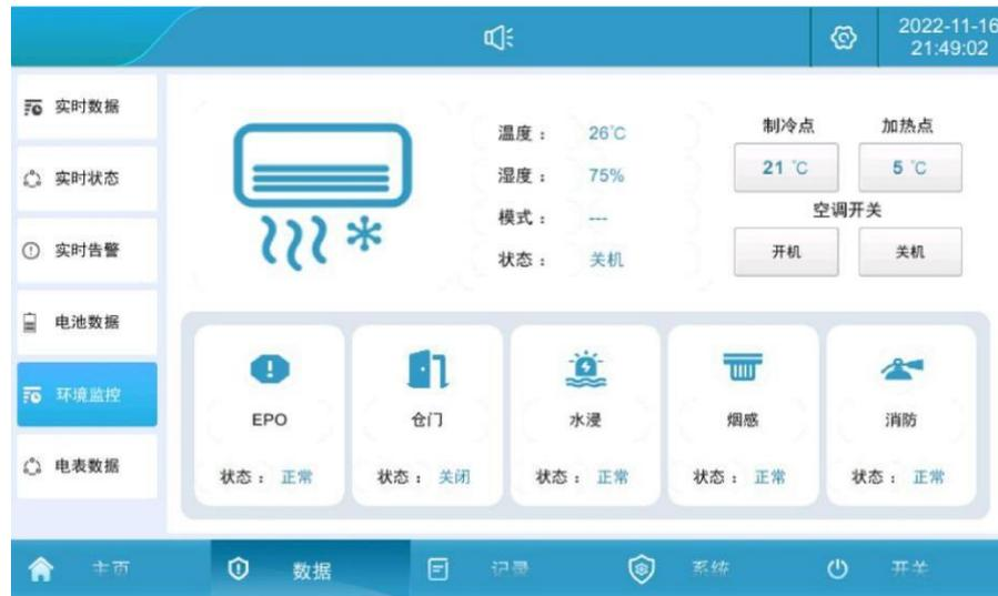
Figure 5.4.6 Environmental monitoring interface
