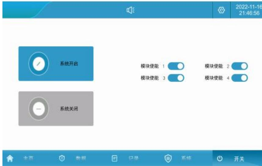
Figure 5.2-2 Power on/off interface
