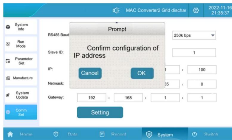
Figure 5.3-3 Address configuration interface
