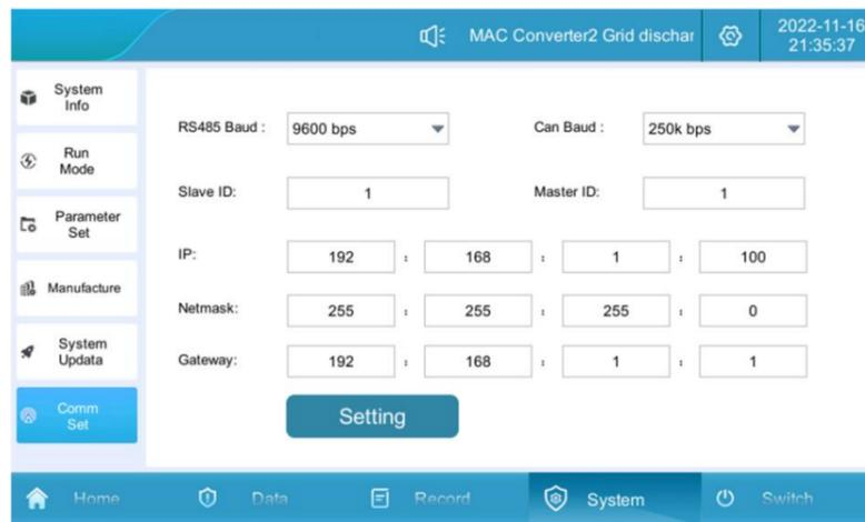
Figure 5.3-2 Communication setting interface
