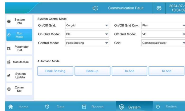
Figure 5.4. 3-4 Peak shaving and valley filling control mode
