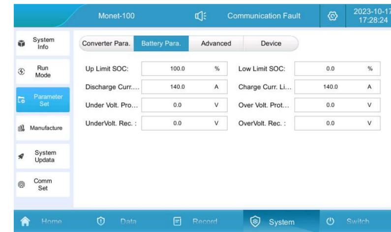
Figure 5.4. 5 Battery charge and discharge setting interface
