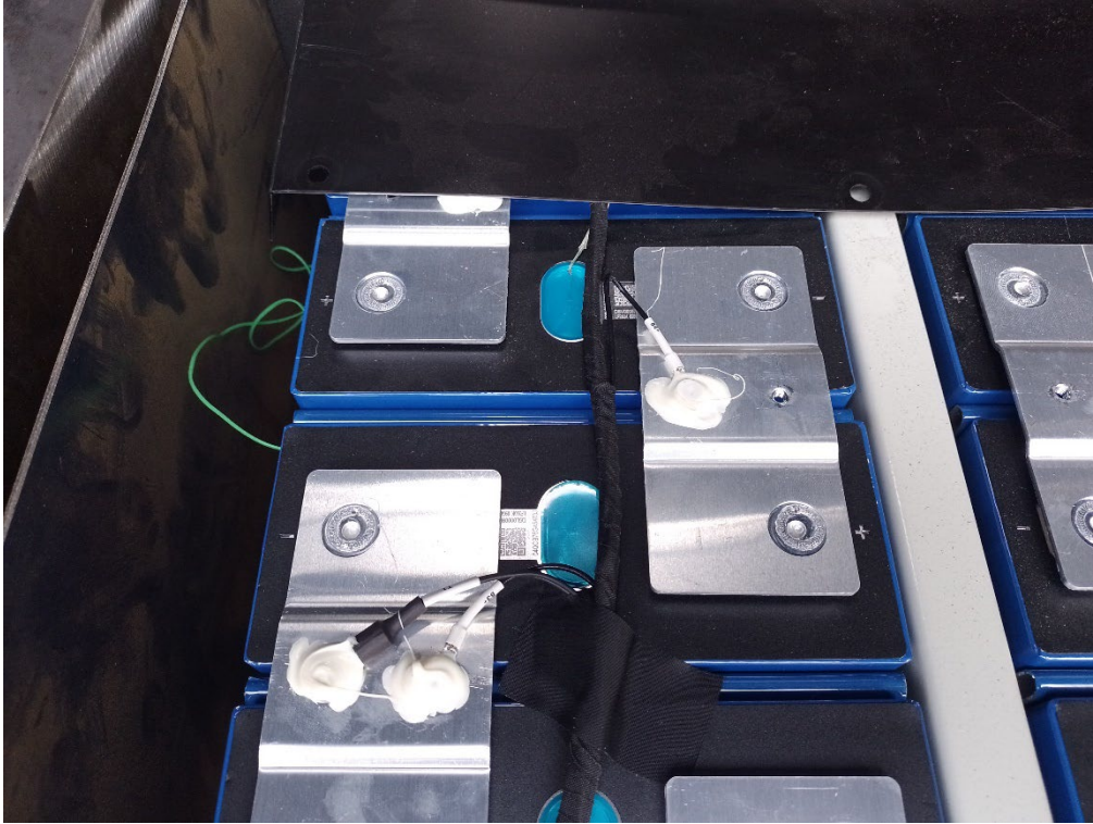
Figure 5 - Sensor location between trigger cell and neighbour cell
