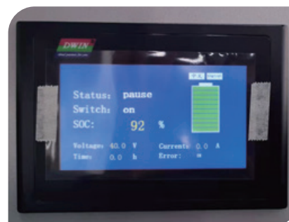
3 电流降为0A，此时LED等闪烁绿灯，等待10秒 The current drops to 0A, at this time the LED flashes green, wait for 10 seconds
