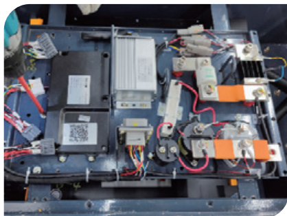
2 拆掉PDU的螺丝并移走PDU Remove the screws on the PDU and remove the PDU
