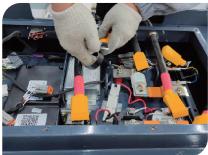
3 拆除动力线并缠上绝缘胶布，移除上盖 Remove power line and wrap insulation tape, remove top cover
