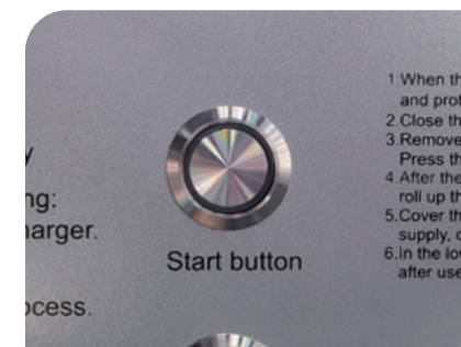
4 若恢复充电，则需按下开始键，便可恢复（无需继续充电则跳过） If you resume charging, you need to press the start button to resume (skip if you don't need to)
