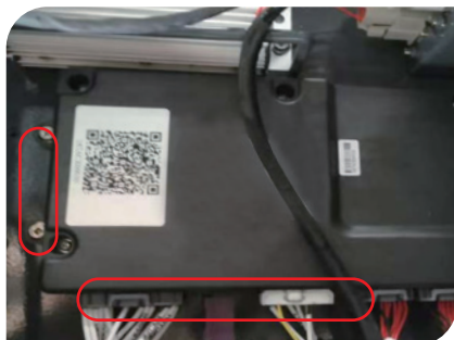
2 拆除BMS上面的连接线束 Remove the wiring harness above the BMS
