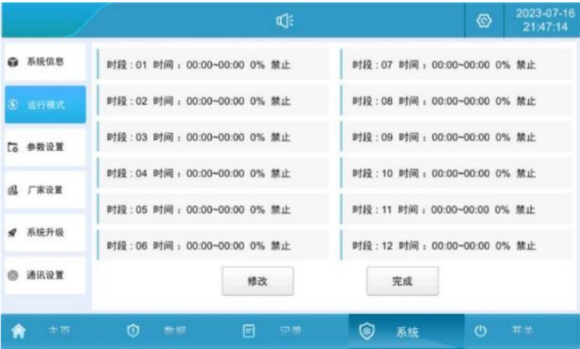
Figure 5.11 Setting interface of peak shifting operation
