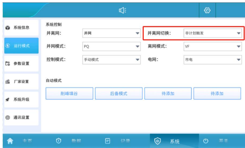
Figure 5.19 Automatic parallel and off-grid switching mode setting interface
