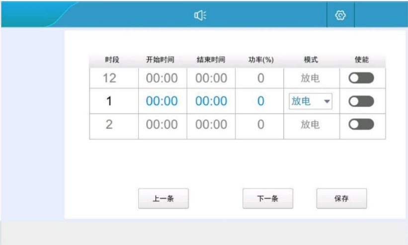
Figure 5.12 Peak load filling time setting interface
