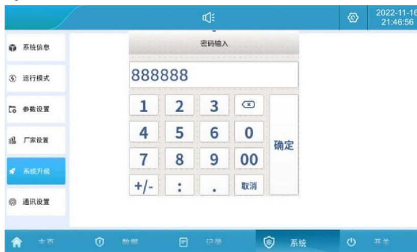
Figure 5.25 Upgrade software password verification
