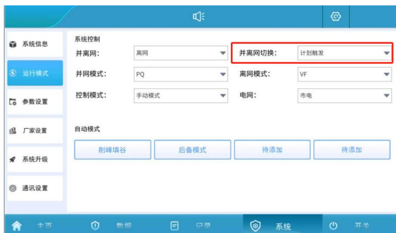
Figure 5.18 Manual and off-grid switching mode setting interface
