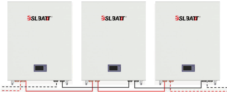
Figure 4-1 Parallel installation diagram
